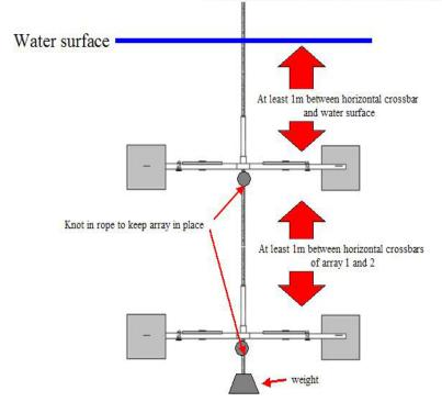
Attach arrays to suitable fixing e.g., rope line between droplines
