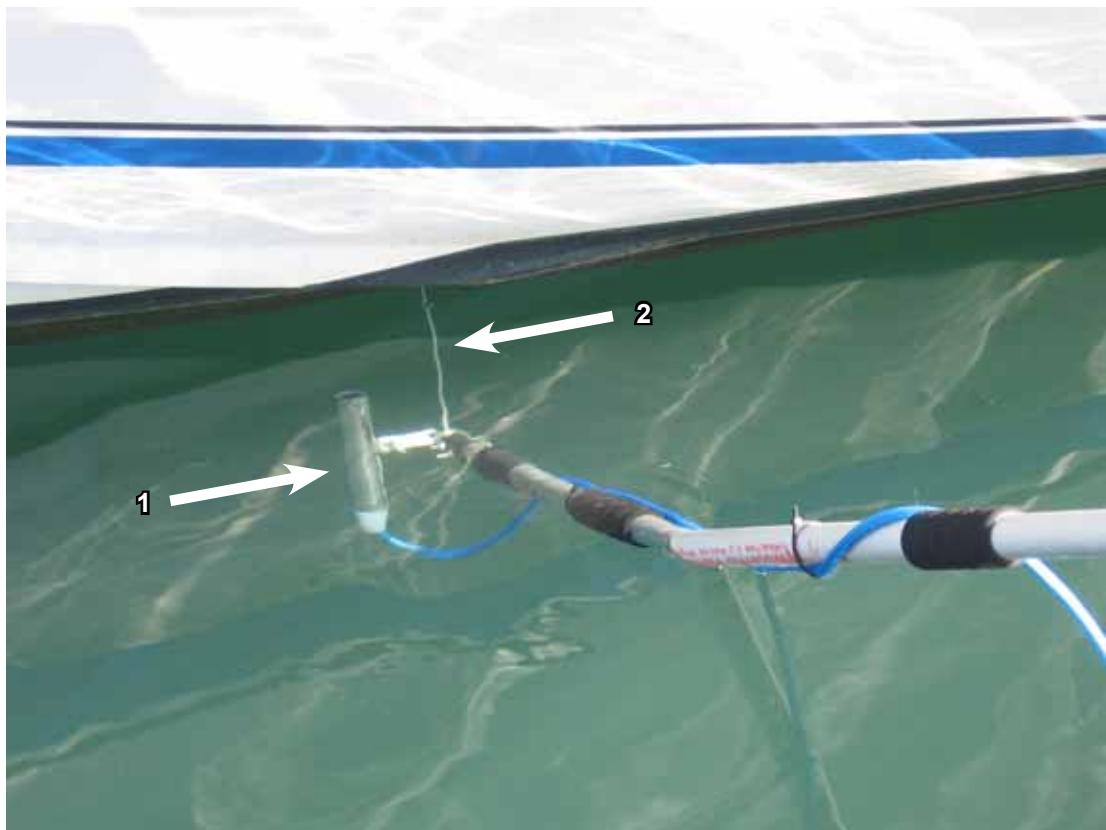
Figure 3. Picture showing the hull camera at work. The arrows are pointing out (1) the camera and (2) the 15 cm spacer used to ensure the camera is at the best focal distance. Photograph Sam Bridgwood.
