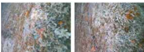
Figure 6. Examples of secondary and tertiary biofouling levels captured by the hull camera on keels.
