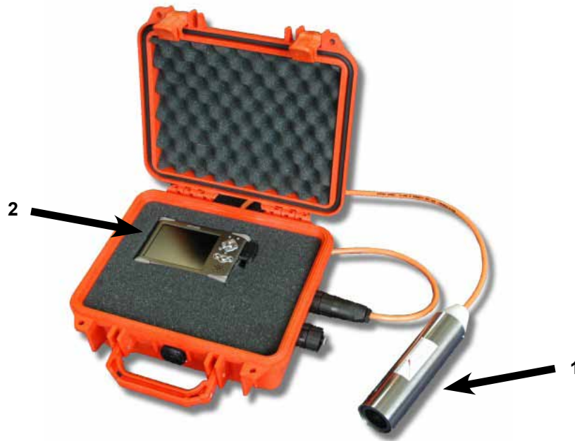
Figure 2. Image showing the video camera (1) (minus the pole) and the video recorder (2) encased in the pelican case. Note the length of the cable is much shorter in this image than was used for the field testing. Image accessed from: http://www.scielex.com.au/products/products_14.html .
