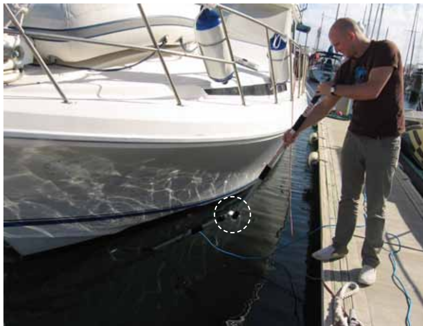
Figure 1. Photograph showing the use of the hull camera from the jetty. The join between the two poles (circle) can be seen, this allowed better access to the hull and other difficult to get to areas e.g. propeller. Photograph Sam Bridgwood.
