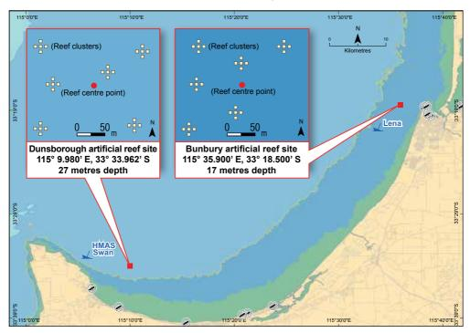
Each artificial reef is made of 30 ten-tonne reinforced concrete modules placed in six clusters in the four hectares reef area.
