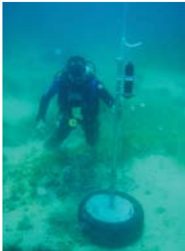
Putting in place the underwater hydrophone part of an acoustic receiver. Photo: Rory McAuley
